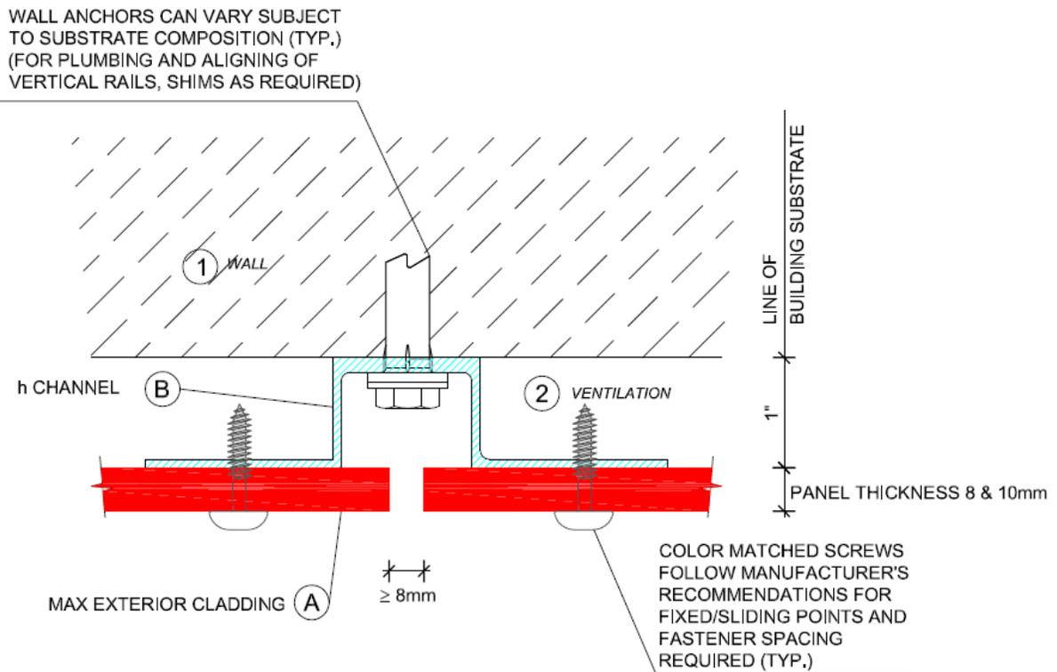
FIGURE 1 – TYPICAL DETAIL – EXPOSED FASTENER SYSTEM
