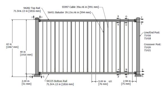
FIGURE 10 - WESTBURY® VERTICABLE SERIES STYLE C80 ALUMINUM RAILING SYSTEM (42" TALL)
