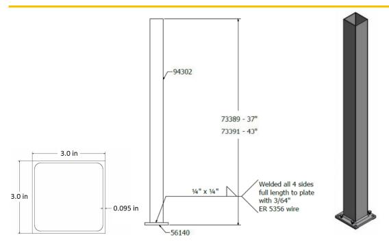
FIGURE 28 – 3" SQUARE ALUMINUM SUPPORT POST ASSEMBLY
