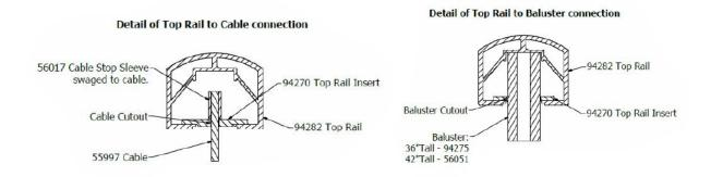
FIGURE 35 - WESTBURY® VERTICABLE SERIES C80 TOP RAIL PROFILES
