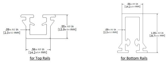
FIGURE 17 - VERANDA SERIES RUBBER INSERTS FOR GLASS INFILL
