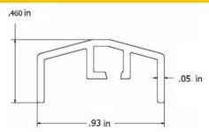
FIGURE 18- LIBERTY PVC INSERT FOR TOP AND BOTTOM RAIL
