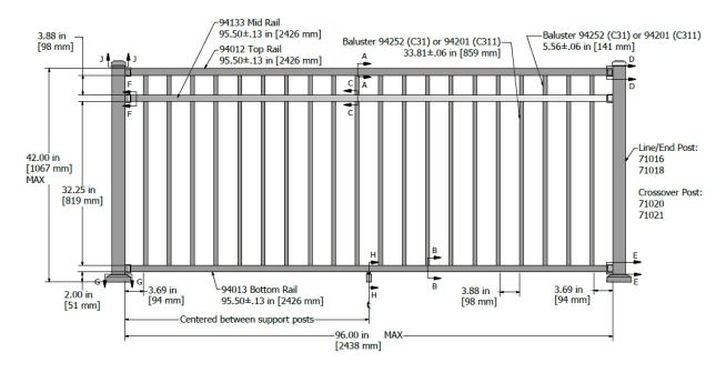
FIGURE 4 - WESTBURY® RIVIERA SERIES STYLE C31/C311 ALUMINUM RAILING SYSTEM
