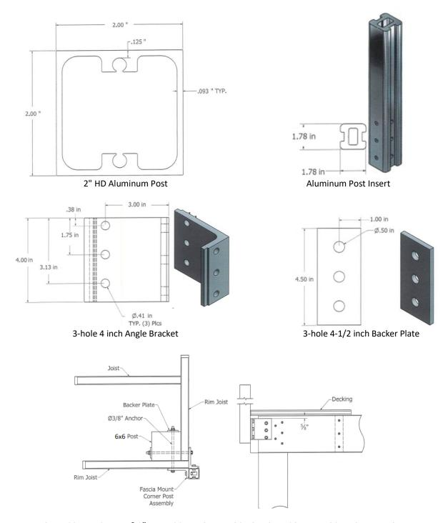
FIGURE 33 – WESTBURY® 2" HD FASCIA MOUNT POST OUTSIDE CORNER POST INSTALLATION
