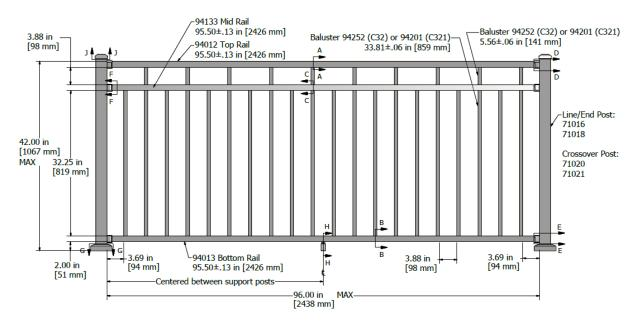
FIGURE 5 - WESTBURY® RIVIERA SERIES STYLE C32/C321 ALUMINUM RAILING SYSTEM
