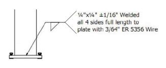
FIGURE 26 - 4X4 ALUMINUM POST ASSEMBLY
