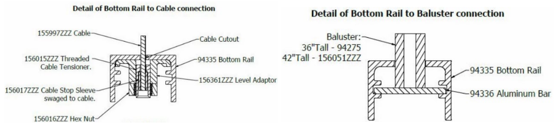
FIGURE 36 – WESTBURY® VERTICABLE SERIES C80 BOTTOM RAIL PROFILES
