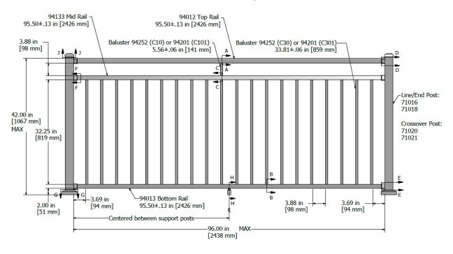
FIGURE 2 - WESTBURY® RIVIERA SERIES STYLE C30/301 ALUMINUM RAILING SYSTEM
