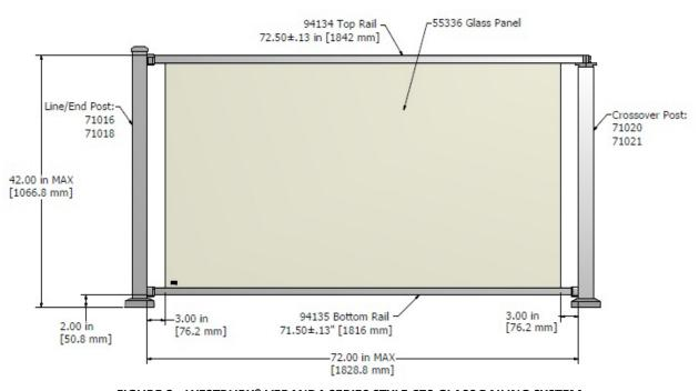
FIGURE 8 - WESTBURY® VERANDA SERIES STYLE C70 GLASS RAILING SYSTEM
