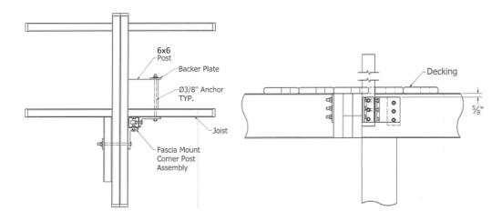
FIGURE 32 – WESTBURY® 2" HD FASCIA MOUNT INSIDE CORNER POST INSTALLATION
