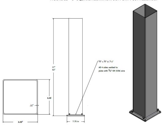
FIGURE 29 – 6" SQUARE ALUMINUM SUPPORT POST ASSEMBLY
