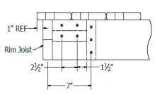
FIGURE 30 – STRUCTURAL WOOD FRAMING 2" POST MOUNT Limited to IRC and FBC Residential
