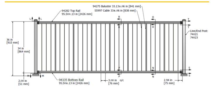
FIGURE 9 - WESTBURY® VERTICABLE SERIES STYLE C80 ALUMINUM RAILING SYSTEM (36" TALL)
