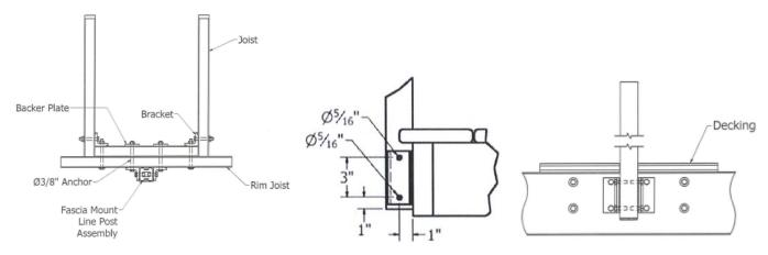
FIGURE 31 – WESTBURY® 2" HD FASCIA MOUNT LINE POST INSTALLATION Limited to IRC and FBC Residential
