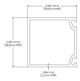
FIGURE 34 - SCREEN RAIL NON-STRUCTURAL POST
