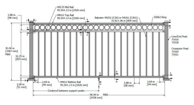
FIGURE 3 - WESTBURY® RIVIERA SERIES STYLE C30R/C301R ALUMINUM RAILING SYSTEM
