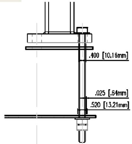
Plate Installation Configuration
