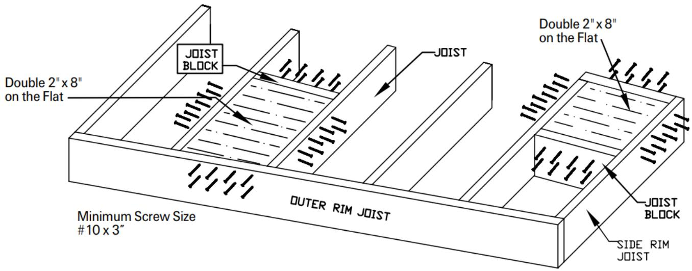
FIGURE 10 – BLOCKING DIAGRAM
