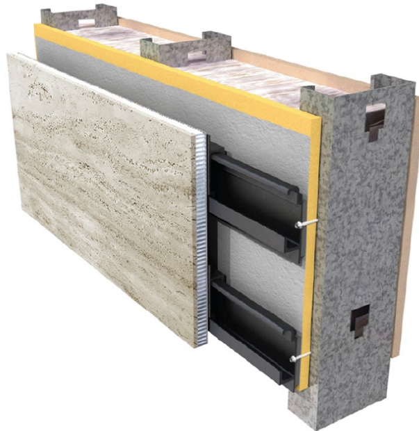
Figure 4 – Typical ALLCOMB Panel Assembly
