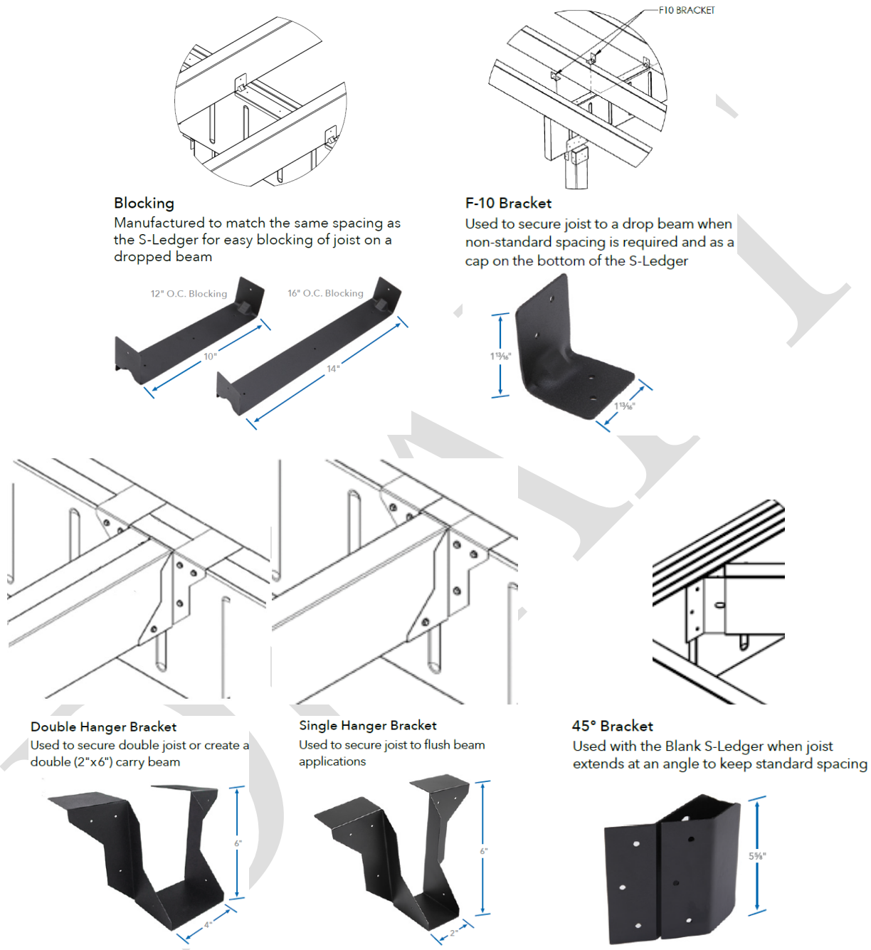
FIGURE 9 – JOIST TO BEAM CONNECTION
