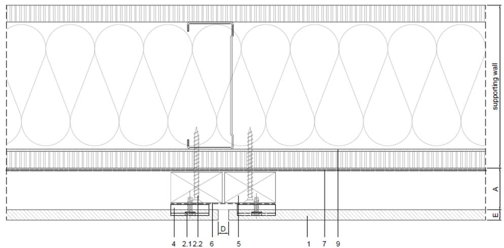
Figure 12 – Vertical Joint – Siding System
