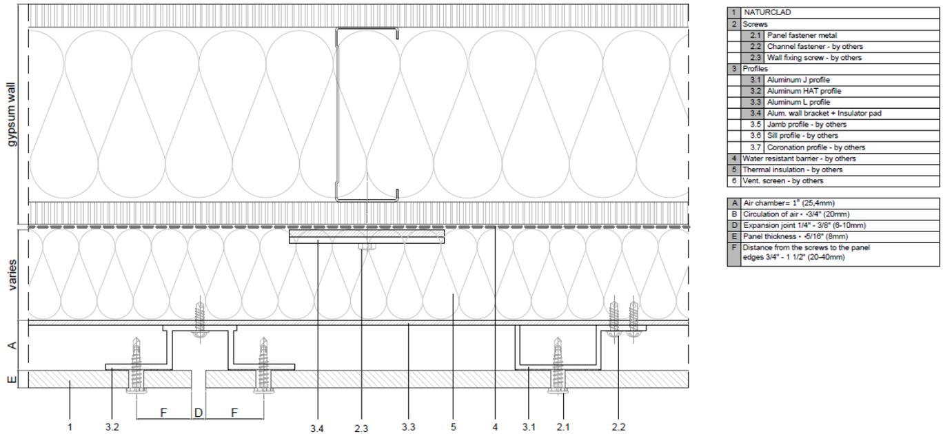
Figure 6 – Typical Installation – Vertical Joint – Aluminum J and Hat Channel, Exposed Fastener
