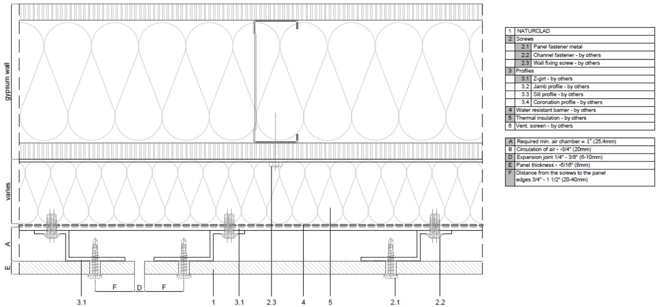
Figure 2 – Typical Installation – Vertical Joint – Z-girts, Exposed Fasteners
